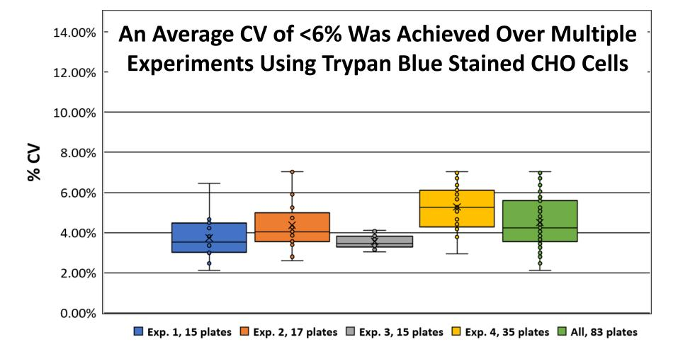
• Multiple users were able to yield an average plate to plate variability for Trypan Blue stained CHO-S cells of less than 6% CV • A total of 1,992 individually loaded samples (83 plates) were counted and analyzed in 70 minutes
