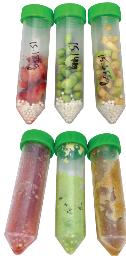
Figure 1 Produce Samples Pre and Post Homogenization. 15 g samples of strawberry, soybeans, and apples were homogenized on the Bead Ruptor Elite with 15 g of ceramic beads in 30 seconds.
