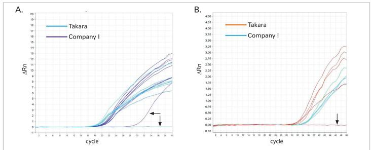
Figure 1. Amplification plots for 28S rRNA (A) and PTGES (B) from individual CP-A cells. The black arrows indicate no template controls.
