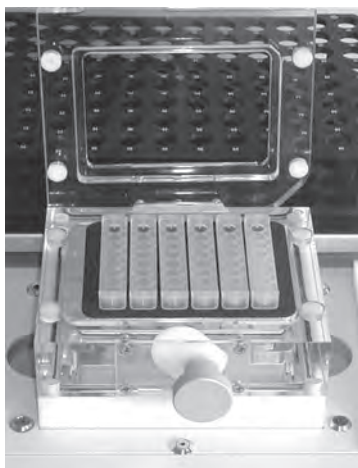
Figure 6: NucleoSpin® Plasmid Filter Strips inserted into Column Holder B placed in the manifold top on the BioRobot® 9600. The lid will press down the strips into the gasket to seal the vacuum chamber.
