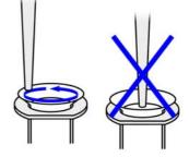
Allow the column to empty by gravity flow. The column does not run dry.
