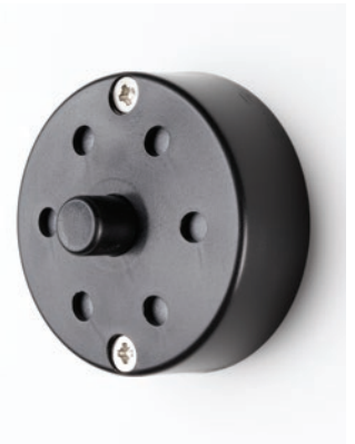
Heated air vent with ice-cleaning plunger prevents vacuum formation, allowing the door to be quickly opened throughout the day
