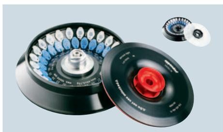
**Rotor for 48 × 1.5/2.0 mL tubes** spins up to 18,210 × *g*/12,700 rpm (FA-45-48-11\*/\*\*\*; Order no. 54277 540.081). Also available with basic plastic lid (F-45-48-11\*\*\*\*; Order no. 54277 550.041).
