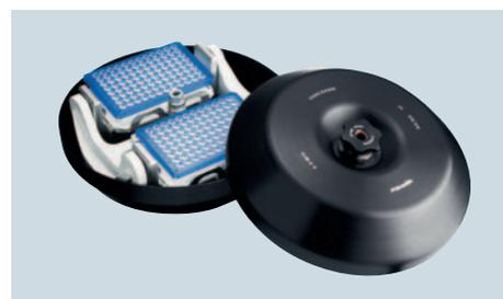
**2-place swing-bucket rotor for MTP, PCR and deepwell plates** of up to 29 mm height; speed up to 2,204 × *g*/4,680 rpm. (A-2-MTP; Order no. 5427 700.005).
