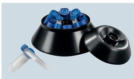
**6 × 15/50 mL conical tube rotor** accommodates 12 × Vacutainer, 6 × 15/50 mL conical tubes. Max. speed of 7,815 × *g*/7,830 rpm (F-35-6-30; Order no. 5427 716.009, includes adapters for 15 mL and 50 mL conical tubes).
