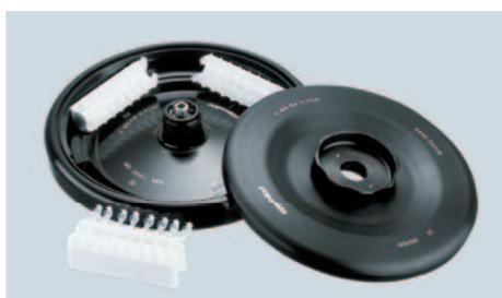
**8 × PCR strip rotor** with removal adapters that can be used as a pipetting rack; maximum speed is 13,543 × *g*/11,800 rpm (F-45-64-5-PCR; Order no. 5427 714.006, includes adapters).
