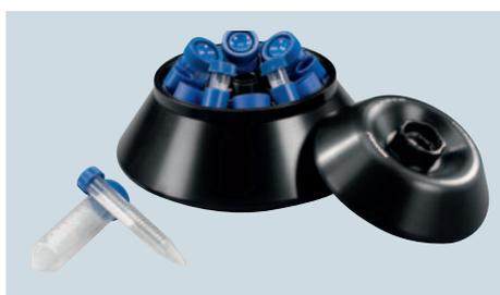
**6 × 15/50 mL conical tube rotor** accommodates 12 × Vacutainer, 6 × 15/50 mL conical tubes. Max. speed of 7,815 × *g*/7,830 rpm (F-35-6-30; Order no. 5427 716.009, includes adapters for 15 mL and 50 mL conical tubes).
