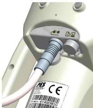
Connect the charger to the mains power supply (voltage 100 to 240 VAC+/- 10%, 50-60 Hz, 700mA). The charger supplies a voltage of 15 V cc, 2A.
