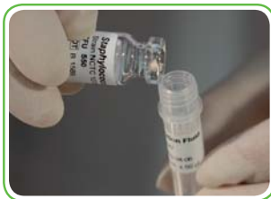
1. Tip the BioBall into BioBall Re-Hydration Fluid, replace the cap, wait 30 seconds
