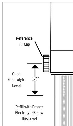
*Always use the appropriate fill solution for your pH electrode. Typically, single junction pH electrodes use the [HI7071](#) electrolyte solution (3.5M KCl + AgCl), while double junction pH electrodes use [HI7082](#) electrolyte solution (3.5M KCl).*
