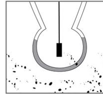
Over time, particles during routine measurement can contaminate the sensor tip.
