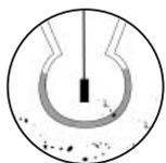
**Why** – Deposits can form on the electrode during use, coating the sensing glass. This can lead to erroneous calibrations and readings.
