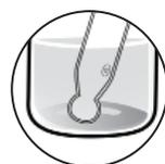
**Why** – Both the pH sensing glass and reference junction need to be completely immersed in order to function properly.
