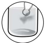
**Why** – Wiping the pH glass can produce a static charge which interferes with the pH reading of the electrode.
