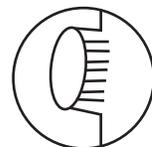
**Why** – A closed electrode fill hole may lead to slower stabilization times.
