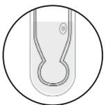
**Why** – Storing in deionized water (DI) causes ions to leach from the glass membrane and reference electrolyte resulting in a slow and sluggish response.
