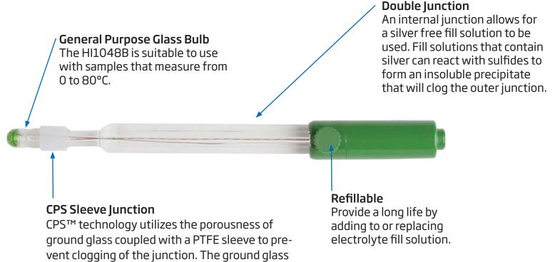
allows proper flow of the fill solution, while the PTFE sleeve repels solids.
