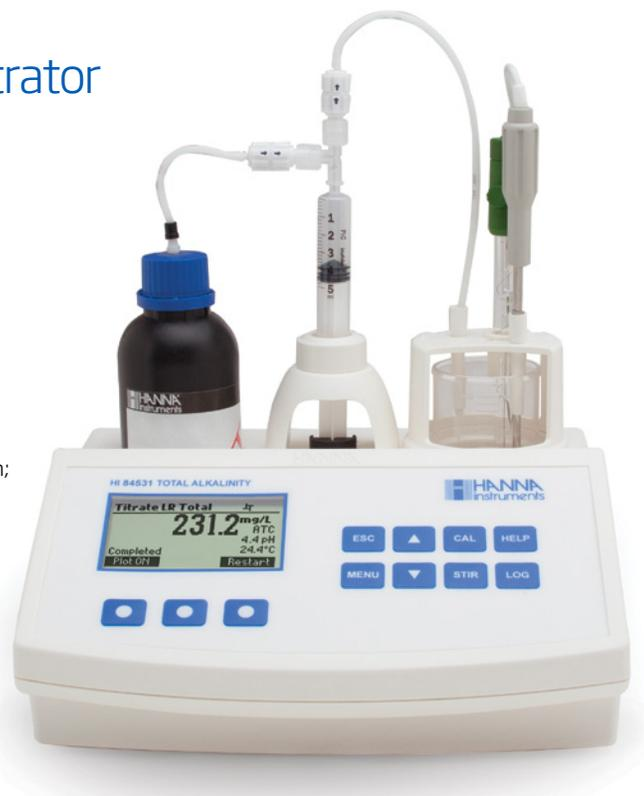
This mini titrator and pH meter is designed for low to high levels of alkalinity. It performs a potentiometric titration with a pH electrode to determine total titratable alkalinity or strong alkalinity in water.
