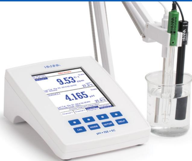
HI5522 is a research grade benchtop meter that features up to eight measurement parameters: pH, mV (for Oxidation Reduction Potential), ISE, conductivity, resistivity, TDS, salinity and temperature.
