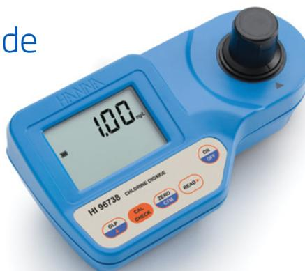
The HI96738C meter measures the chlorine dioxide content in water samples. This meter uses an exclusive positive-locking system to ensure that the cuvette is in the same place every time it is placed into the measurement cell.
