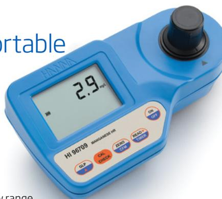
The HI96748C measures the low range manganese content in water and wastewater. The HI96709C measures the high range manganese content in water and wastewater.
