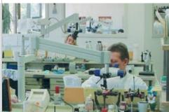
A fiber-optic cold-light illuminator integrated into the Stemi DV4 SPOT Stereomicroscope always illuminates the complete object field of view.
