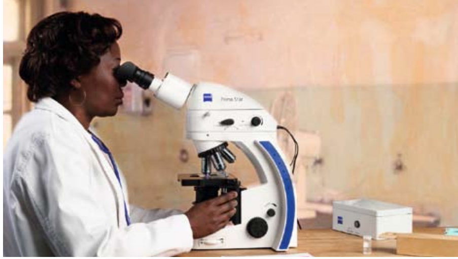
The LED-based fluorescence microscope Primo Star iLED simplifies the microscopic analysis of pathogens
