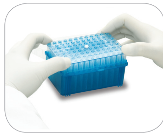
Secure plate by firmly pressing on all four corners of the alignment plate.
