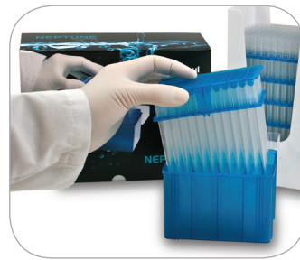
Hold the alignment card away from the side posts and insert the tips into your empty tray.
