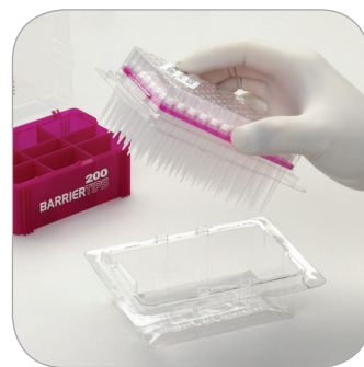
Remove alignment plate from the packaging base by gripping alignment plate using the upper portion of the clamshell packaging.
