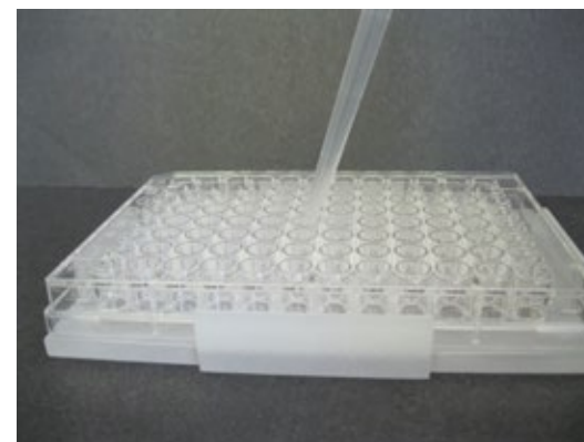
Fig. 4: Use the 96-well holding drive to hold 3D cultures as you add and remove liquids
