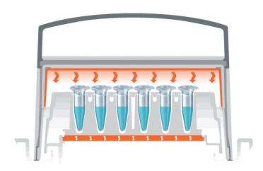
Fig. 1: Cross section Eppendorf ThermoTop
