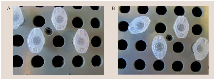
Fig. 3 A and B: Eppendorf ThermoMixer C / Eppendorf SmartBlock 1.5 mL: 1.5 mL Eppendorf Safe-Lock Tubes filled with 1 mL water. The tubes were heated to 56 °C for 10 min without the use of the Eppendorf ThermoTop (A), and with the use of the Eppendorf ThermoTop (B)
