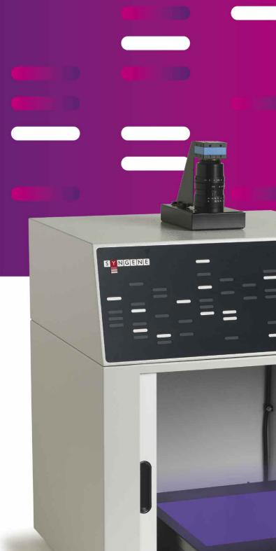
The InGenius<sup>3</sup> uses a high performance 3m pixel camera. The darkroom assembly is easily connected to a PC. GeneSys image acquisition software quickly and easily enables images to be captured, archived and edited if required.
